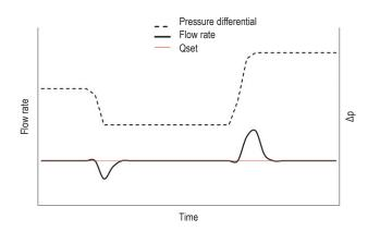
The set flow rate value ( $Q_{set}$ ) is achieved and kept constant by adjusting the valve opening, thus ensuring that the system being controlled is independent of pressure variations.
