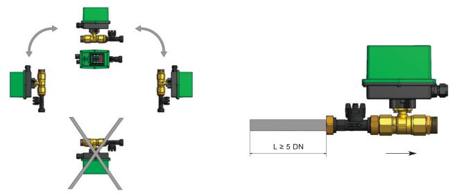
The device can be installed on both the flow line and the return line.
