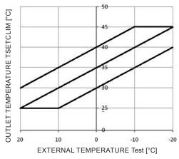
The setpoint temperature is constrained to a temperature range of [+25°C; +45°C].
