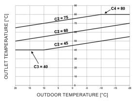
Two parameters, C3 and C4, limit the curves to a minimum and maximum temperature value respectively.
