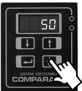
Press the D-ON/OFF button: the display will show the real-time temperature detected by the probe placed on the outlet pipeline. The system is now operating.
