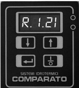
The installed software version immediately appears on the display (see example in the picture).
