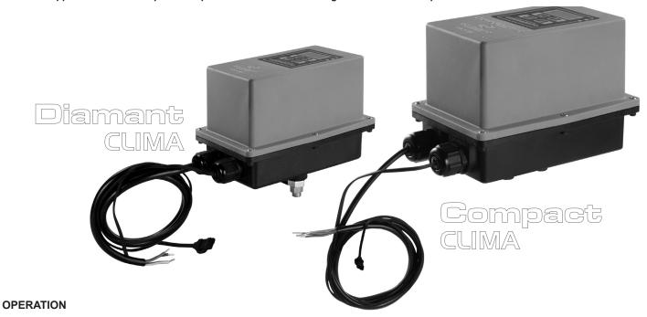
The **Diamant CLIMA** and **Compact CLIMA** actuators are controlled microprocessor which allows to intercept or deviate the fluid according to the temperature detected by the probe. The semiconductor temperature probe, connected to 80 cm-long cable, detects the temperature of the pipeline. The value at which the servo-motor actuator shall start and the operation it shall perform are set on the integrated digital display.
