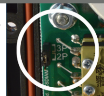
PARTICOLARE JUMPER ALL IN ONE DETAIL OF THE "ALL IN ONE" JUMPER
